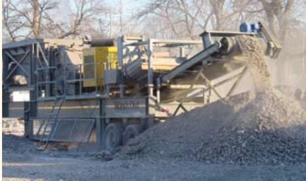
**Fig. 9 Crushed concrete from other sources can serve as recycled aggregate. Photo: Portland Cement Association.**
