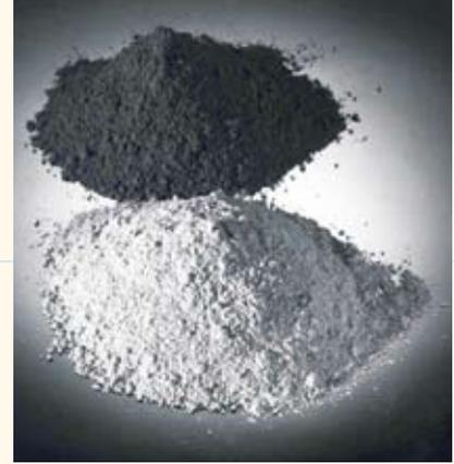
Fig. 8 [c] Silica fume (top) and white silica fume (bottom)
